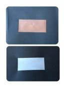
10mm x 20mm areas removed processing rates >1cm<sup>2</sup> / s for Cu AND >2cm<sup>2</sup> / s for Al.
